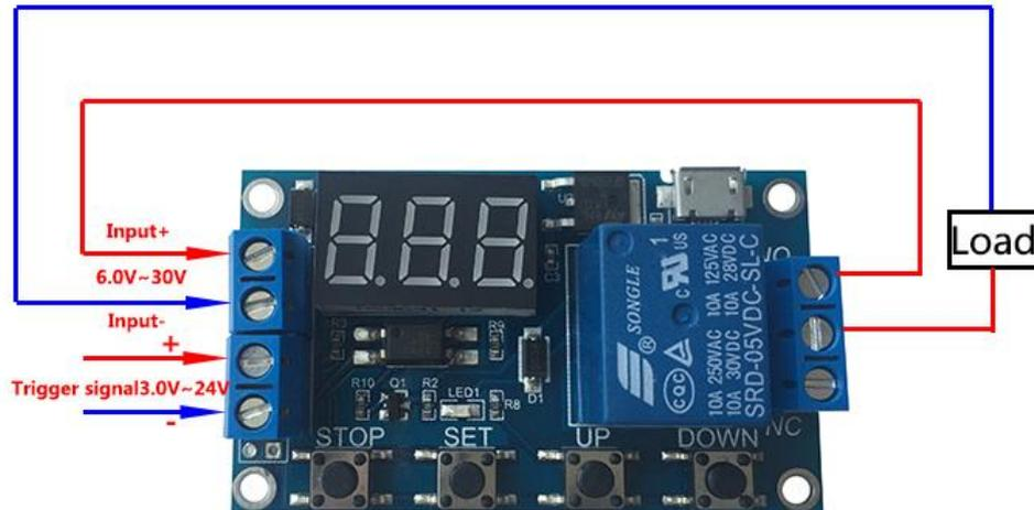
Share a power supply wiring diagram
